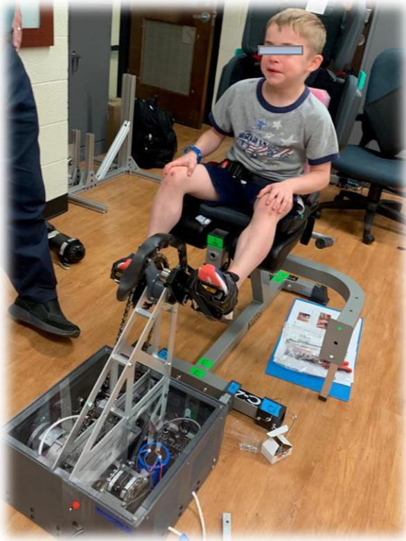
Feedback controllers track cadence and adjust level of motor-assistance in real-time
